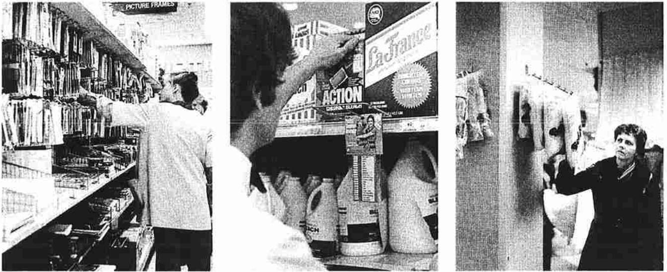
Figure 25-3. Point-of-purchase display hangers must be located in such a way that the human eye cannot contact them (such as shown at left where both the upper and lower shelves project beyond the hangers). Shelf hangers must be safeguarded if they project into the aisle ( center ). Locating projections above eye level is another safe method ( right ).
